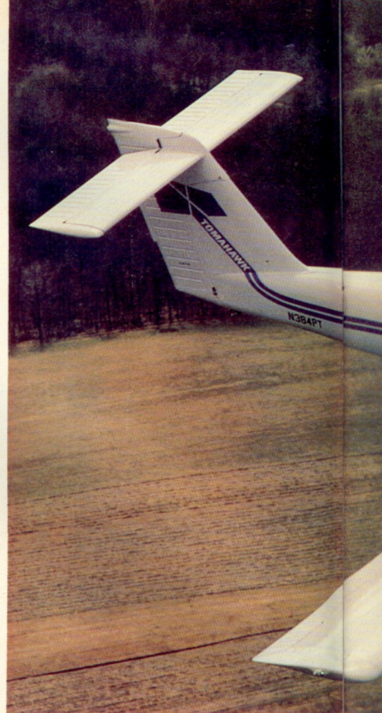
Long, spatula-like wing is a new NASA-technology airfoil, offering flight characteristics unlike Piper's previous trainers.
